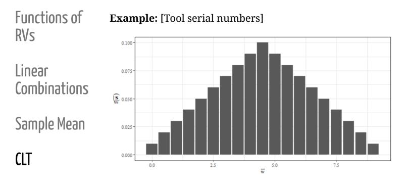
Comparing the two distributions, it is clear that even for a completely flat/uniform distribution of W and a small sample size of n = 2, the probability distribution of W looks more bell-shaped than the underlying distribution.
